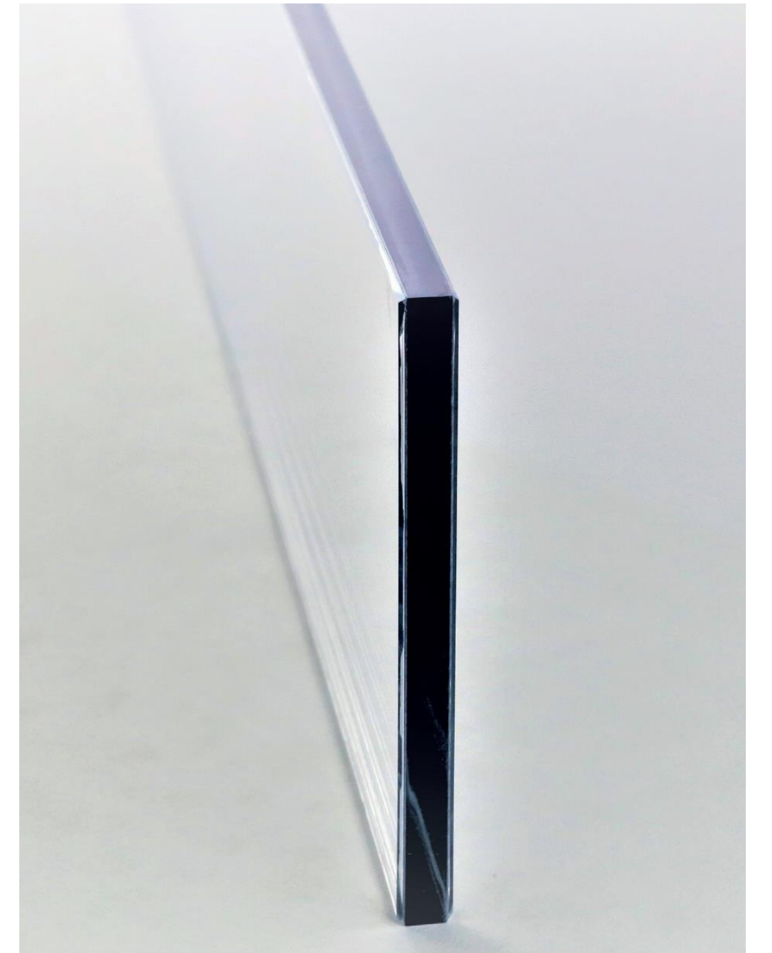
Figure 1: Glass-plastic-composite panel structure (build-up and view)
