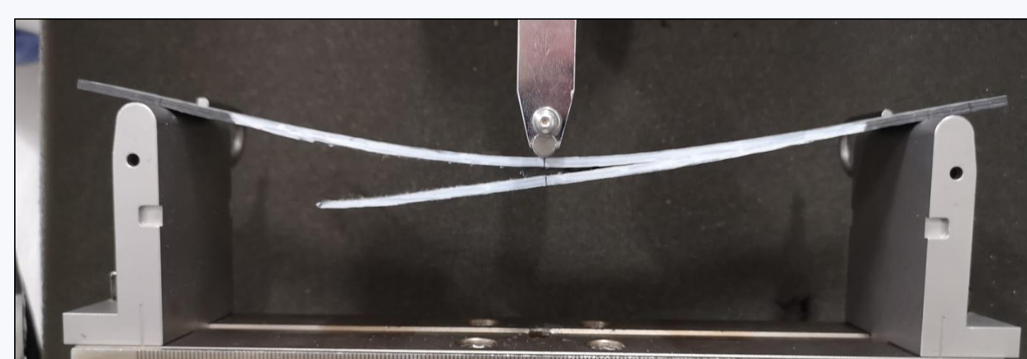
Skin-stiffener debonding / final failure
