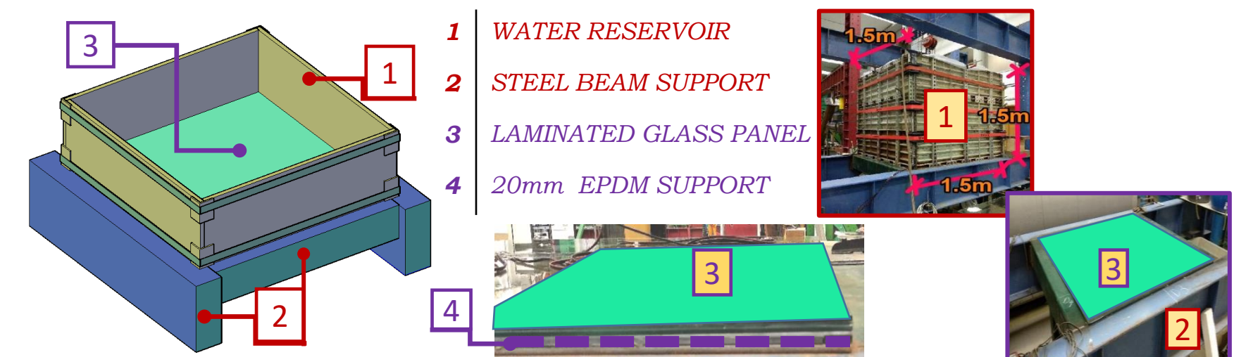
Fig. 2 – Experimental campaign Simple Supported Laminated Glass Panels
