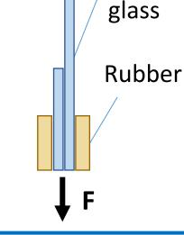
**Adhesive** Sampl strength  $\tau$ Failure formlabs 😿 (Mpa) **UV-curable** Stock break 48,99 Clear Resin 52,15 **Adhesive** (Ø 4mm) 39,22 **Adhesive** 39,60 **Adhesive** Silanized 56,00 Stock break 42,22 Stock break 47,84 Stock break Stock break 53,27 47,97 Adhesive Stock break 53,13 10 36,65 11 Adhesive Adhesive Strength  $\tau$  = 43,12  $\pm$  6.61 MPa
