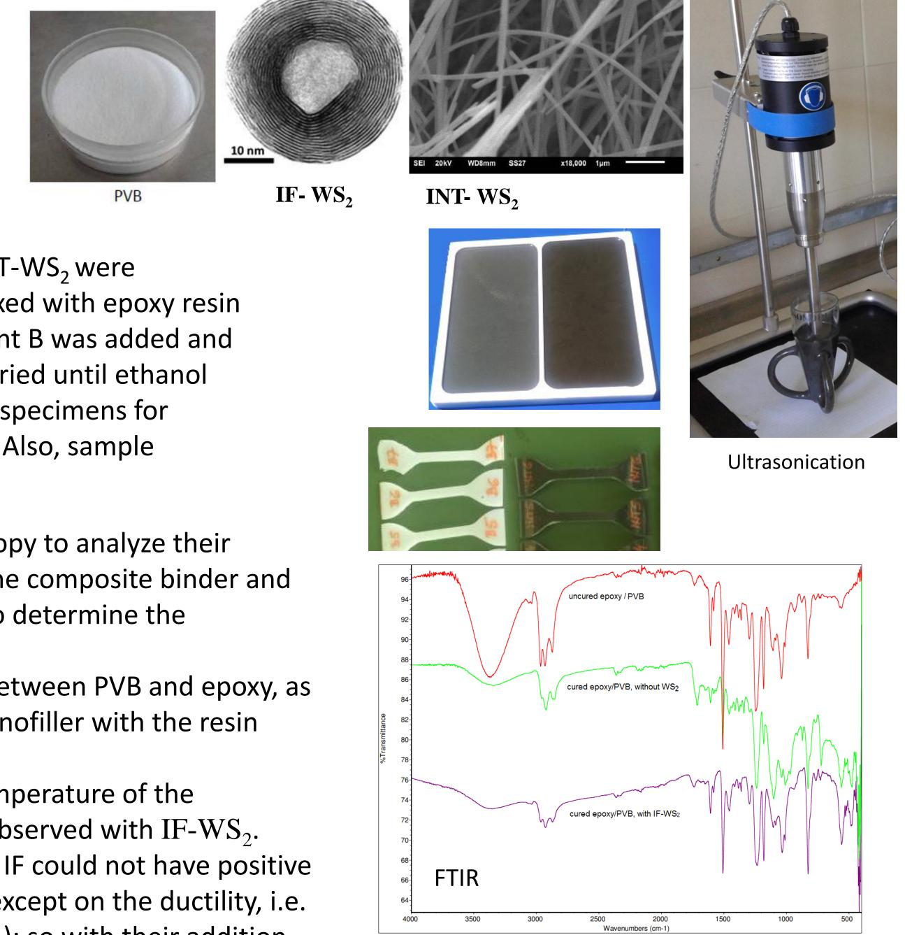
PVB was dissolved in ethanol in which IF-WS<sub>2</sub> or INT-WS<sub>2</sub> were ultrasonically dispersed; then this solution was mixed with epoxy resin component A, and after homogenization component B was added and mixed. The mixture was cast into flat moulds and dried until ethanol evaporated. Thick film samples were obtained and specimens for mechanical tests and other analyses were cut out. Also, sample PVB/epoxy without WS<sub>2</sub> was made.
