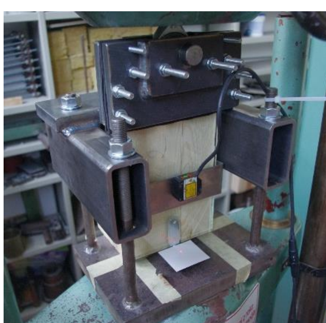
Fig. 9. Timber-glass point joint shear test
