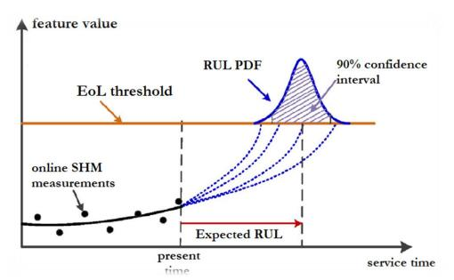
In the Figure the concept of SHM-based prognostics is highlighted.
