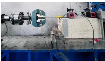
Figure 1: Pull-out test setup for concrete blocks strengthened via EBR technique
