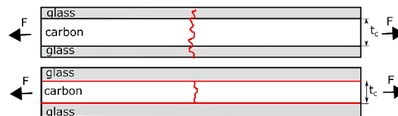
Figure 1: Failure modes in bonded hybrid glass/carbon layers. (i) crack through the whole specimen thickness; (ii) crack in the carbon layer followed by single delamination.
