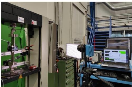
**Figure 1: Testing set-up - DCB quasi-static tests.**
