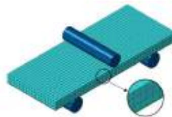
Figure 2: FE numerical model of 3PB experimental setup
