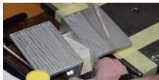
Figure 2: Applying the adhesive
