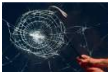
Figure 1: Fracture pattern of glass fitted with ASF system after impact
