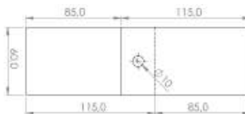
Figure 1: SLS specimen dimensions
