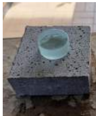
Figure 2: Concrete-Glass Shear Specimen
